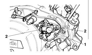
Fit the carburettor oil feed pipe (1) and ensure that there are no air bubbles. Also fit the line that feeds oil to the pump (2), and then fasten both pipes with the related clamps.
