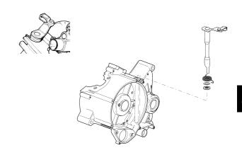
Clutch lever oil seal drift: 8201530
