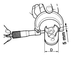
▲ CAUTION: The maximum allowable ovalization is 0,10mm. Change the cylinder and piston assembly every time this value is exceeded.
