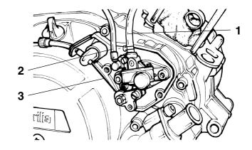
Loosen the two fixing screws (1), take off the oil pump (2), and then remove the O-ring.
