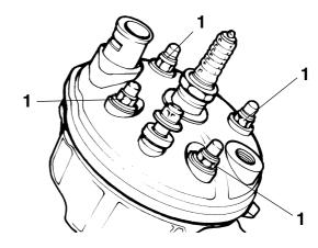
Tightening torque: 14 ÷ 16 Nm
