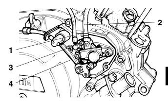
Replace the oil pump cover and fasten it using the two fixing screws.
