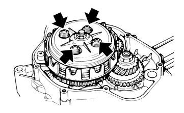
▲ CAUTION: When disassembling the clutch, pay special attention to the relative positions of the components to ensure that they are reassembled properly.
