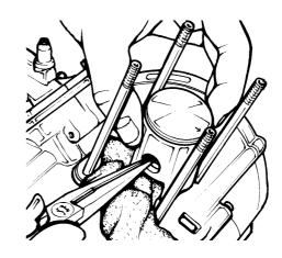
Fit a new gasket on the cylinder, the cylinder, a new central O-Ring, new O-Rings in the studs, a new O-Ring on the head, the head (remove any carbon formation first), lock diametrically opposed nuts (1) in an even manner, checking that the O-Ring on the head has been correctly positioned.
