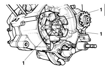
Fit the rotor and lock it.
