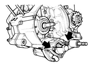
Tightening torque: 5 Nm
