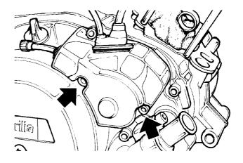
After removing the clamp, detach the line that feeds oil to the pump (1) and stop it to prevent the oil from coming out. Detach the pipe that feeds oil from (2) the pump to the carburettor.
