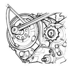
Remove the flywheel magneto rotor using an extrator with suitable dimensions, screw it in the rotor's threaded seat, keep it into place with a spanner and act on the central screw with a 17 mm spanner.
