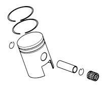
Ensure that the piston rings are in perfect condition and that the clearance between the ring ends is as shown in the table below.
