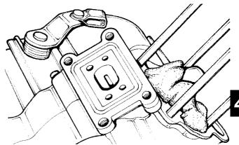
Fit the intake manifold and fasten it with the fixing screws after inserting the clutch cable bridge. Tighten the 4 screws in a progressive and crossed way.
