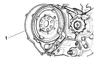
Tightening torque: 1 ÷ 2 Nm
