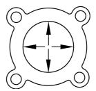
Repeat the measurement at several points along the barrel between the cylinder upper surface and the exhaust port.
