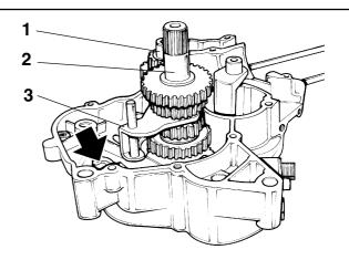
Fit the desmodromic shaft (1). Fit the fork in the sliding of the 2nd and 3rd gear along with its guide pin.
