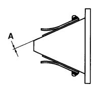
Measure the height of the reed valve stops (A). If it is outside the tolerance range, replace the stops. Reed valve stop height: 9 mm  $\pm$  0.3 mm.
