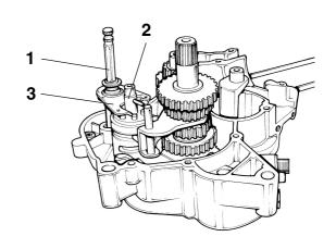
Also check that, when the desmodromic shaft is positioned on the 2 nd gear, the cam rollers are at equal distances from the fork lips. If not, gently distort the spring ends until the desired situation is obtained.
